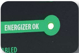
Energizer On and OK indicator (green LED)
