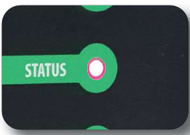
Status indicates fence overload or internal energizer fault (red LED)
