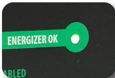
Energizer On and OK indicator (green LED)
